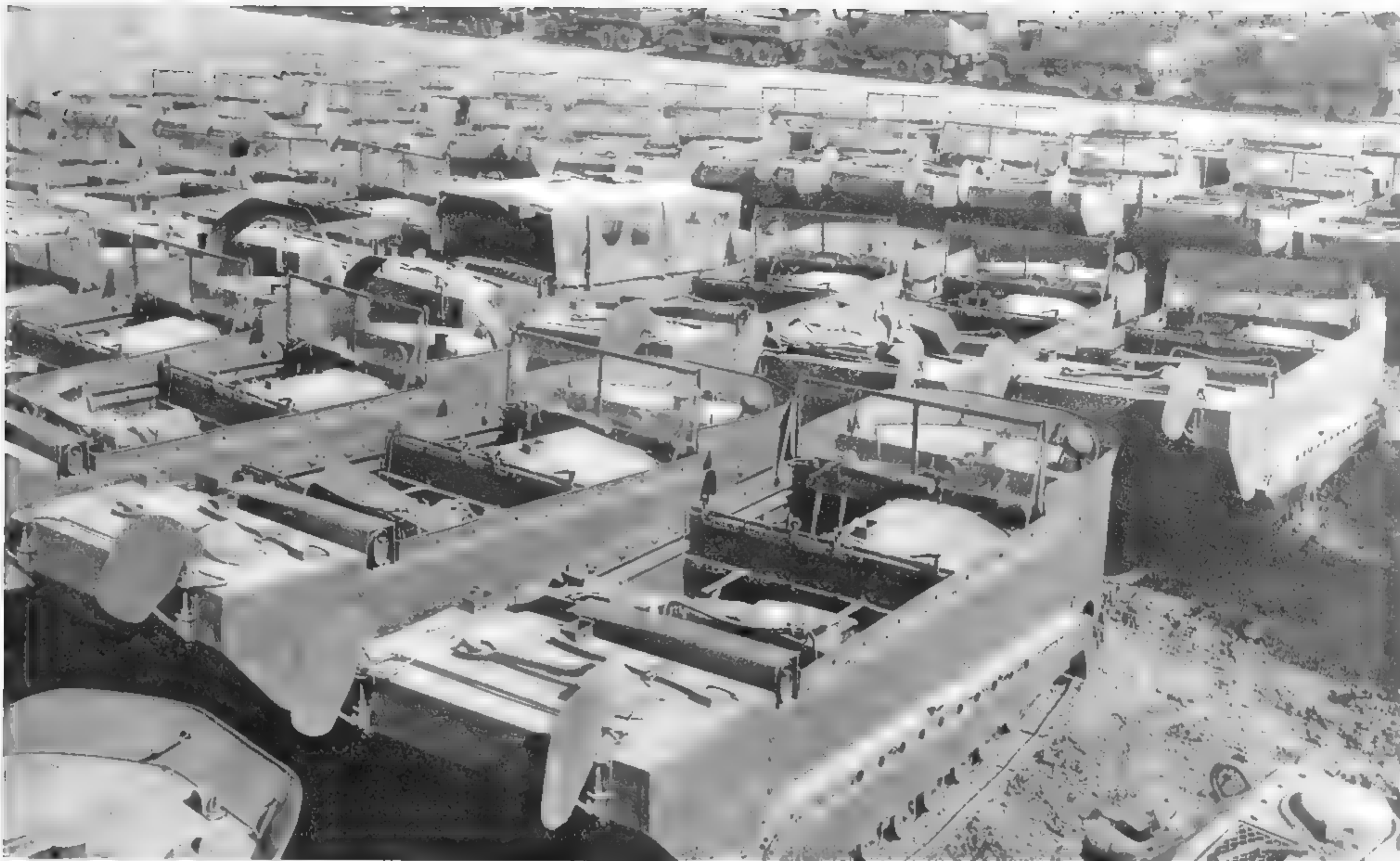
This group is undoubtedly a Weasel collector's dream. This Signal Corps photo of a group of M29Cs was taken at Manila, the Philippines. Some of them have their surf shields swung up, between the stowed and usable condition, and one has its canvas cab cover fitted. All of them have their pioneer tools in place, and in the foreground we can see the cover next to the driver's seat. Under that cover is the Studebaker Champion engine. (National Archives and Records Administration photo)
